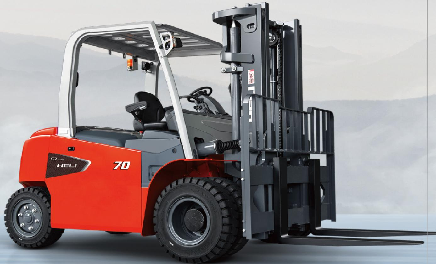
The truck is a continuation of HELI family style and creates a new concept of electric forklift through easy exchange between lead acid battery power and lithium battery power
